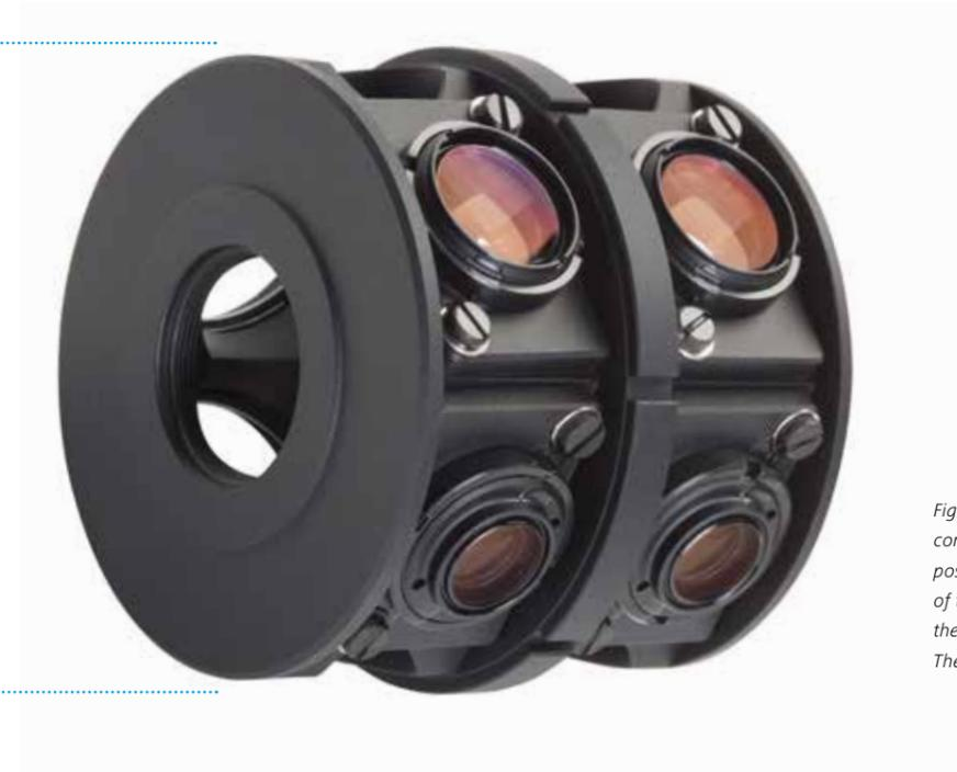
Figure 1.6: A five-step magnification changer is composed of a turret with two telescopes and one position without a lens. Depending on the position of the magnification changer in the optical path, there are different magnification factors. The factor in the lens-free position is 1.
