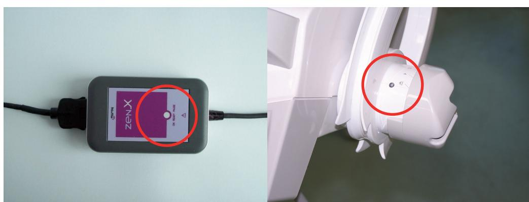
A red light indicates a serious fault for which it is not possible to take the x-ray (the self-diagnosis system detected at start up).
